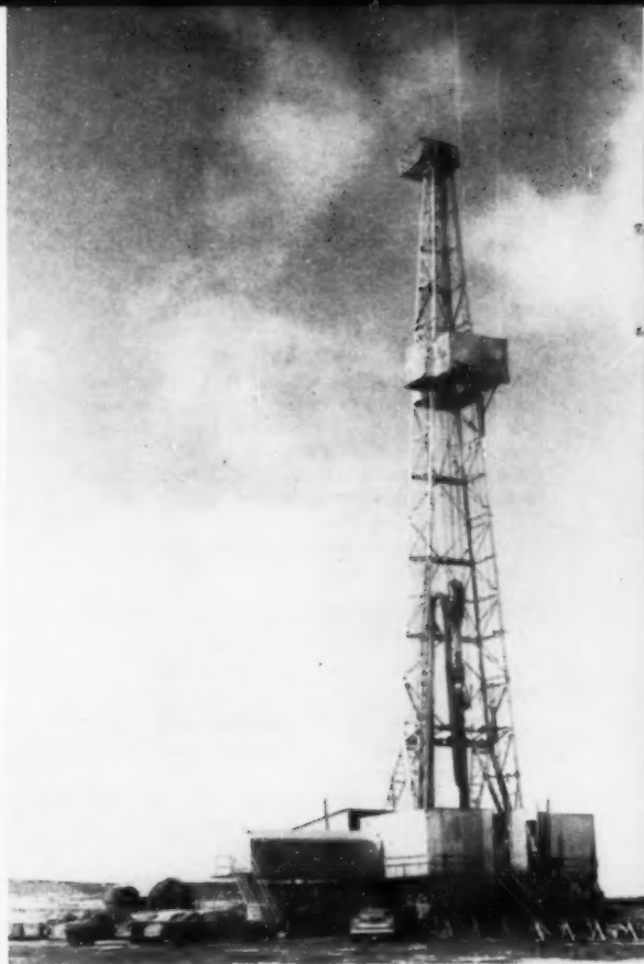
KERR-McGEE'S No. 7 rig, medium size by oil well standards, has 135-foot-high Lee C. Moore derrick.
